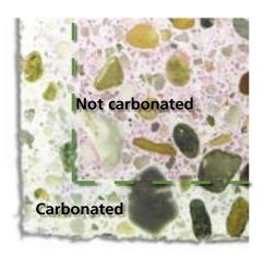
The  ${\rm CO_2}$  emitted in the calcination of limestone is reabsorbed by the calcium present in cement. This reaction takes place within concrete and mortars and is called concrete carbonation.
